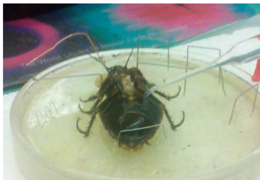
Figure 2. Photograph showing the biofuel cell implanted into B. discoidalis .
